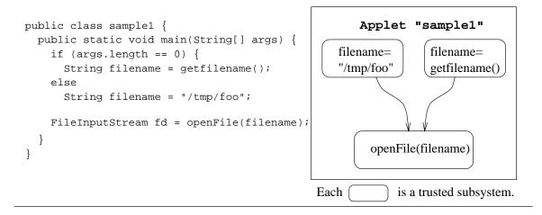
Figure 4.1: Example Flow Diagram and Corresponding Code.
