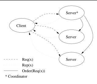
Figure 7: Process and message architecture.
