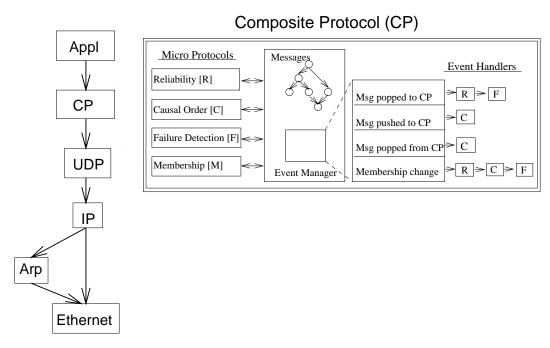
Figure 3.1: Composite protocol within an x-kernel protocol graph.
