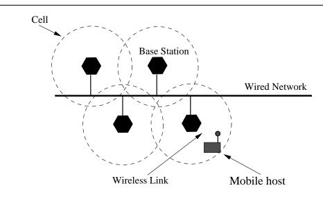
Figure 2.1: Hardware components of a typical mobile distributed system.
