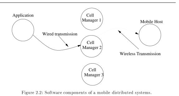
*Cell Manager.* Executes on the base station or on a stationary host controlling the base station. Manages the wireless communication within the cell, forwards routing information to other cell managers, and controls traffic between wired and wireless networks (Figure 2.2).
