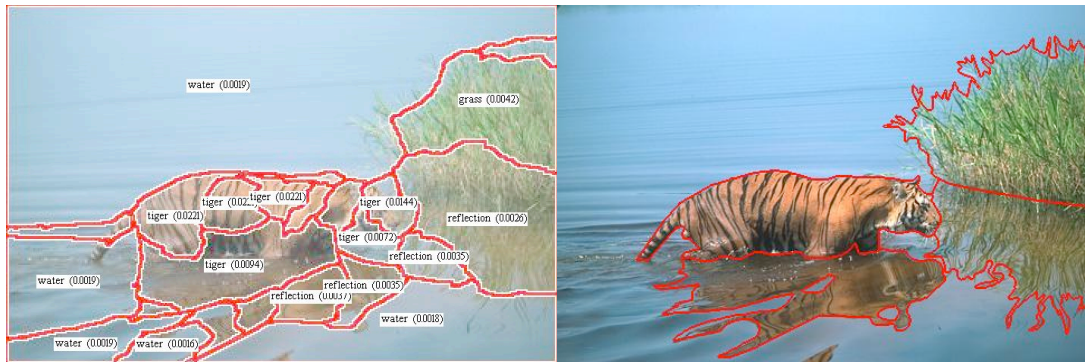
Figure 8. Illustration of mapping of the ground truth data onto experiment specific data. The regions are labeled with the word that would receive maximal score (in parenthesis) under the semantic range scoring method. The machine produced segments (left) are scored as a blend of the underlying ground truth segments (right). The blend is not simple because the vocabulary words need to be connected to one or more ground truth words which may be scored according to how frequent they are (depending on the scoring approach).
